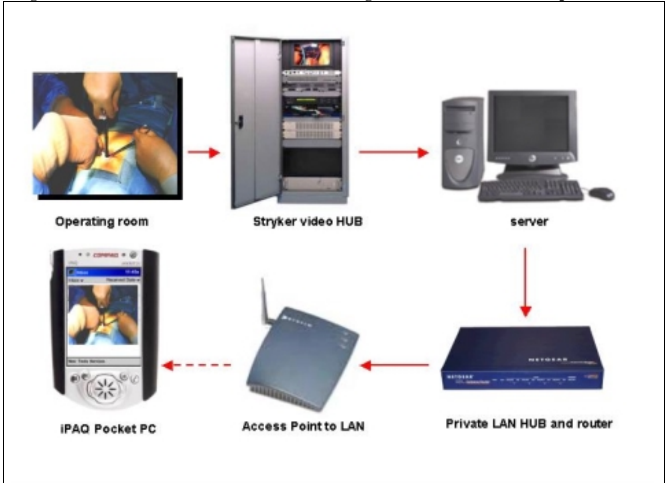
Figure 1: Wireless Transmission of Live Streaming Video to a Handheld Computer
